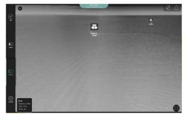
Live images are displayed in the colour and thermal camera view. Detected objects are displayed with a bounding box. If the OSCAR system is able to classify the detected object, an icon is displayed. Clicking on the icon displays more details about the selected target.
